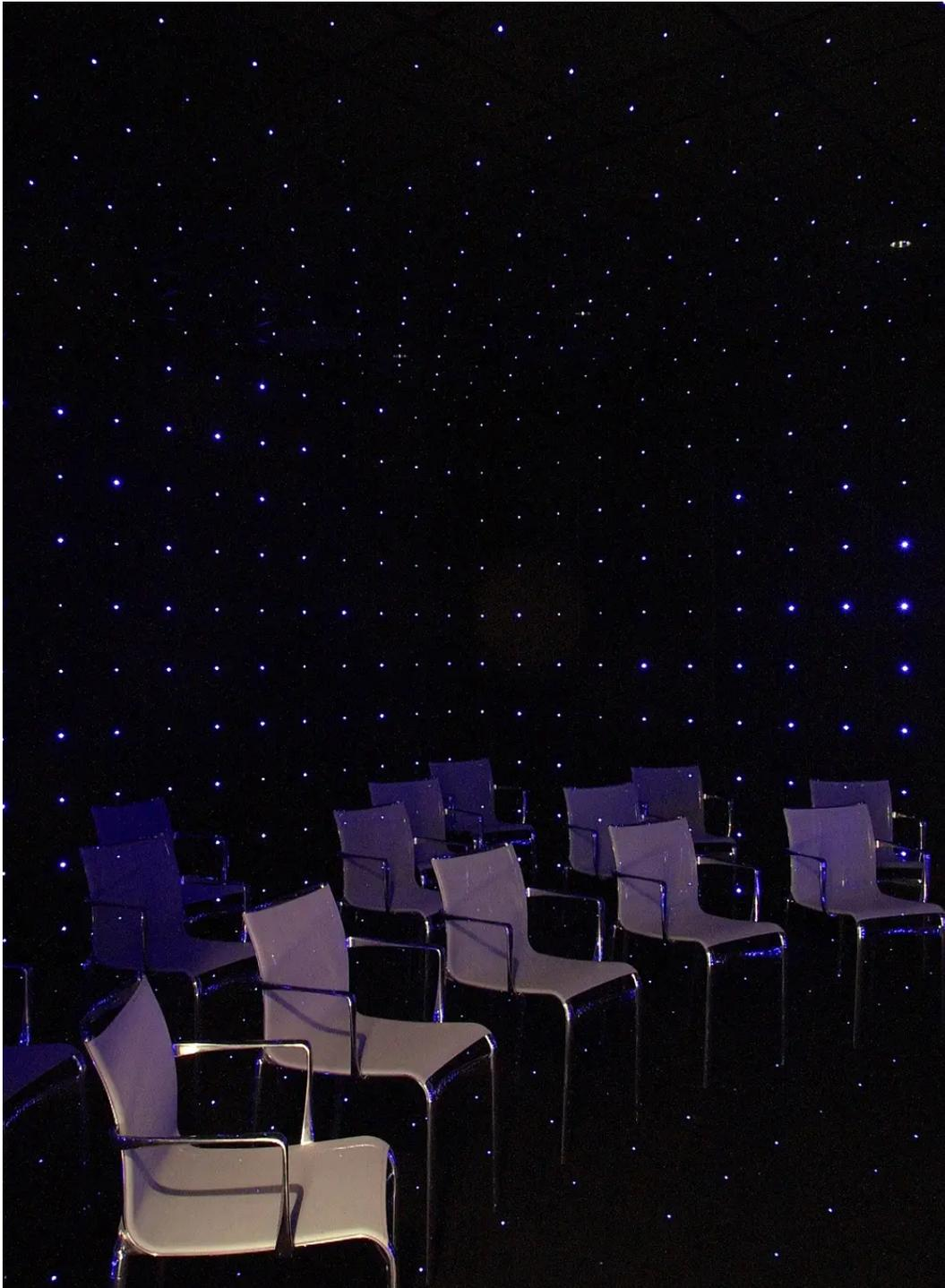
Guides wear a wireless transponder which allows the lighting system to track their position and respond according to where they are in the space. The effect is to create virtual rooms within the main space of the centre.
